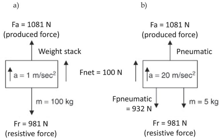
FIGURE 7A Theoretical comparison between a) weight-stack and b) pneumatic resistance (Frost et al. 2010).
