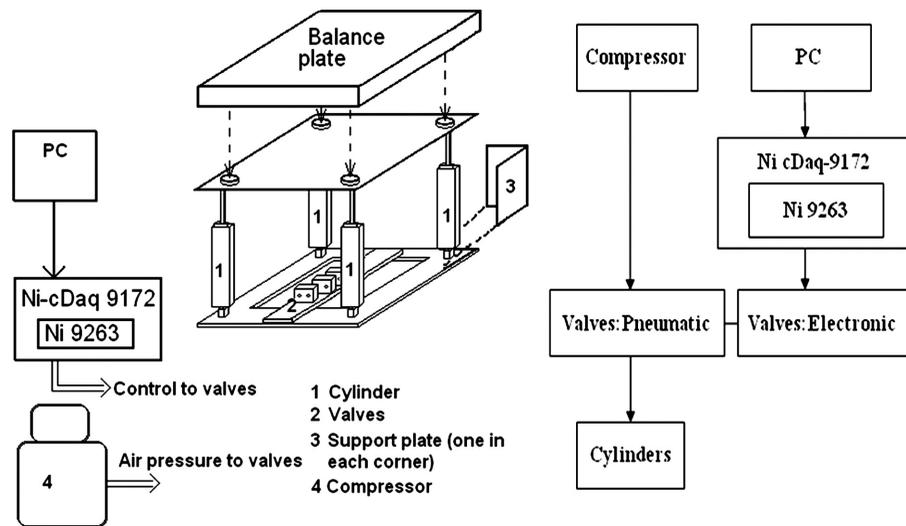
Figure 1. Dynamic balance measurement system and flow chart.
